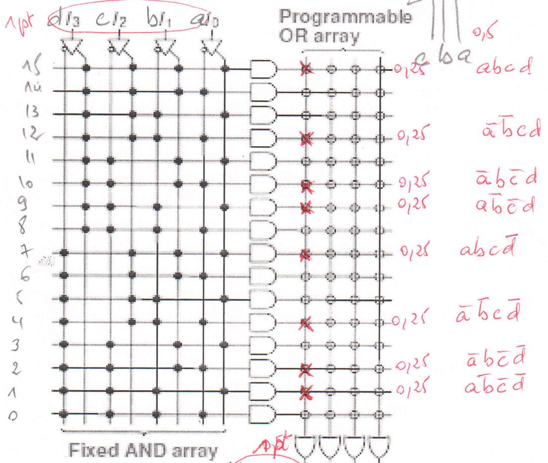
$$\text{Somme} = a\bar{b}\bar{c}(d+\bar{d}) + \bar{a}b\bar{c}(d+\bar{d}) + \bar{a}\bar{b}c(d+\bar{d}) + abc(d+\bar{d})$$
